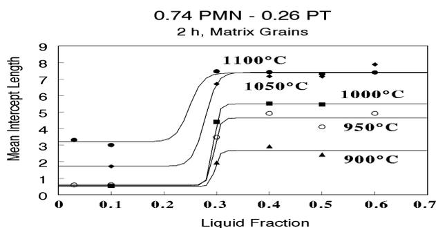
**Figure 1:** The size of matrix grains increases rapidly for liquid fractions about 0.2 and is independent of liquid fraction above 0.3, indicating that growth is not controlled by diffusion through the liquid phase
