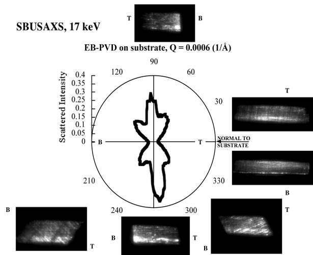
Figure 2: SBUSAXS data at  $Q = 0.0006 \text{ \AA}^{-1}$  versus angle to the substrate-normal for an EB-PVD TBC. SBUSAXS images taken at various sample orientations are also shown where T and B denote the top and bottom of the TBC, respectively.
