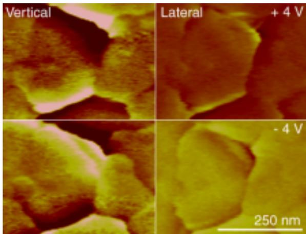
Figure 1 Piezoresponse microscopy shows contrast reversal with changes in the DC bias field applied. The contrast reversal in both the lateral and normal response demonstrates that  $180^\circ$  switching of domains has occurred rather than  $90^\circ$  switching.
