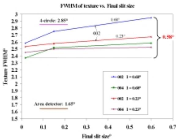
**Figure 2: Texture results from ZnO film processed at 650 °C. Powder diffractometer results are plotted as function of final slit size for various incident slit sizes (I). The 4-circle and area detector results are shown as horizontal lines.**
