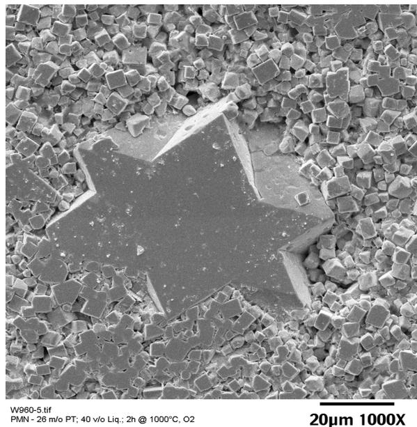
**Figure 2:** Scanning Electron Microscope image of an exaggerated PMN-PT grain in a polished section. Note the reentrant angles on the grain interface which give such grains a growth advantage over the surrounding cube-shaped grains.
