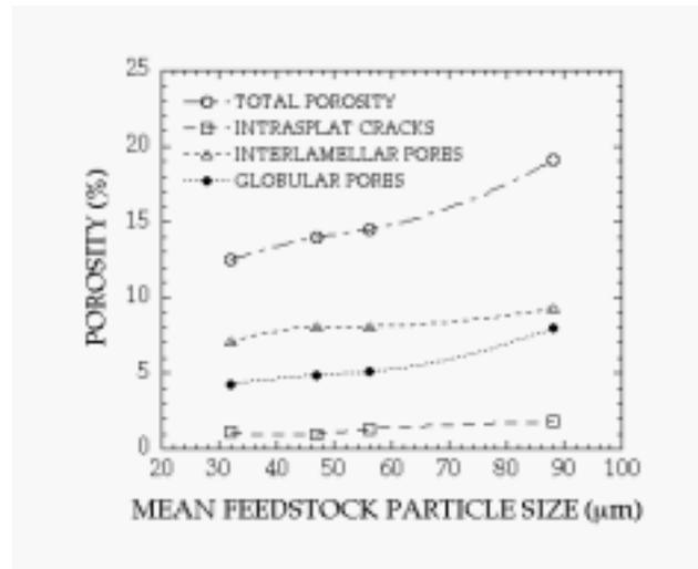
Figure 3: Total and component porosities *versus* mean feedstock particle size. (Total porosity from precision density measurements.)
