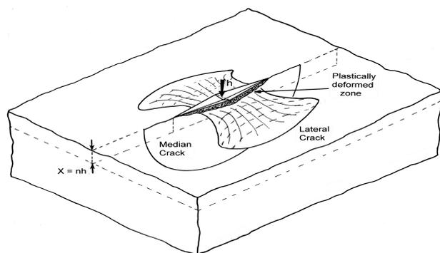
**Figure 1: Lateral crack formation under the Knoop indent**
