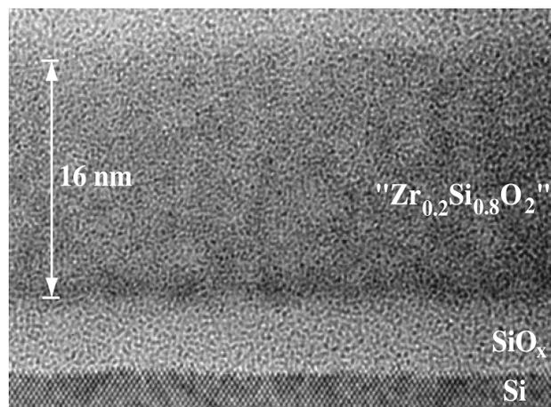
Figure 2: HRTEM image of amorphous zirconium silicate with nominal composition  $Zr_{0.2}Si_{0.8}O_2$ ; the actual composition measured by EDS is close to  $Zr_{0.5}Si_{0.5}O_2$ .
