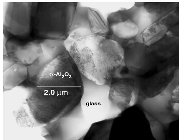
**Figure 2: TEM micrograph of LTCC production device consisting of alpha- $\text{Al}_2\text{O}_3$  particles with sizes ranging up to  $\gg 5 \mu\text{m}$  contained within a continuous glass phase. For this particular device, the glass phase was found to be a calcium-aluminum-silicate, containing various concentrations of Pb, Ti, Na and K.**
