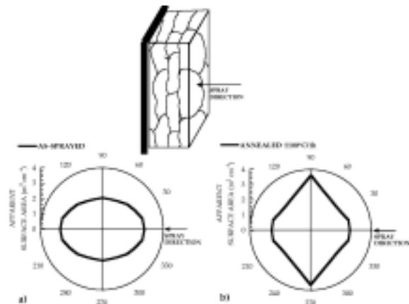
Figure 1: Apparent surface area distributions from NS-SANS studies of a YSZ deposit: a) as sprayed; b) annealed.
