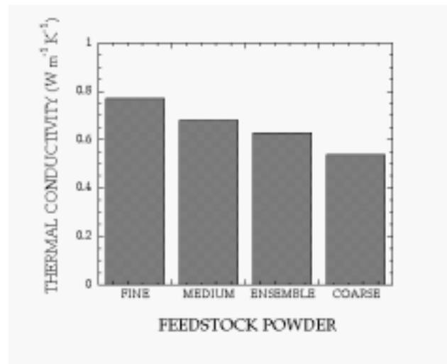
Figure 4: TBC thermal conductivity *versus* feedstock particle morphology.
