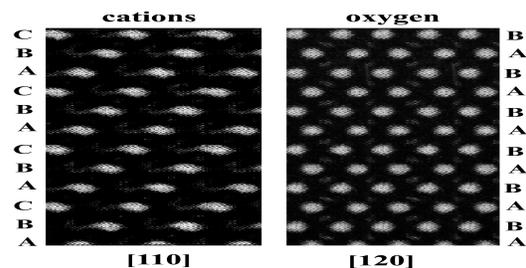
Figure 2: Computer simulated phase contrast images of  $\text{LiNbO}_3$  in both the [110] and [120] orientations. These two projections reveal the stacking sequences of the cation and oxygen layers, respectively, and for the  $\text{Li}_{1+x-y}\text{Nb}_{1-x-3y}\text{Ti}_{x+4y}\text{O}_3$  specimens, revealed that it is not a continuous solid solution, but rather a homologous series of distinct phases.
