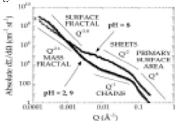
**Figure 1: USAXS data for nanoparticulate zirconia suspensions**
