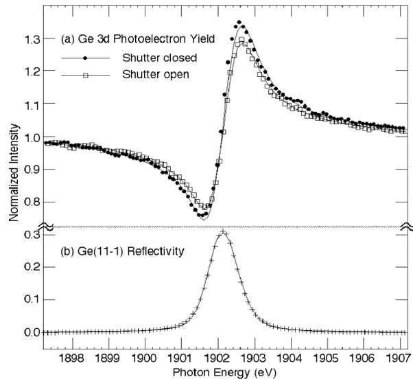
**Figure 1: (a) The Ge 3d photoelectron yield as a function of photon energy around the Ge(11-1) Bragg back-reflection condition. Both the quadrupole-sensitive data, taken with the analyzer shutter closed (filled circles), and the angle-averaged data, taken with the analyzer shutter open (open squares), are compared. The solid lines are the best fits to the data using the dipole-only XSW yield equation. (b) Reflectivity data and best fit.**
