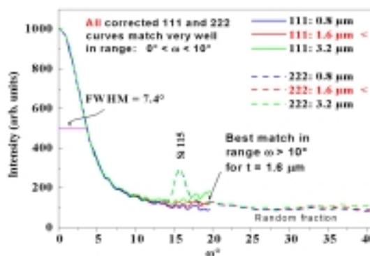
**Figure 1: (111) texture measurements from 1.6  $\mu\text{m}$  thick electrodeposited copper films, measured with 111 and 222 peaks and corrected for thicknesses of 0.8  $\mu\text{m}$ , 1.6  $\mu\text{m}$  and 3.2  $\mu\text{m}$ . Specimens provided courtesy of Semitool Corporation.**
