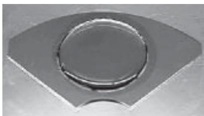
**Figure 2:** Confined lubricant solution on a hard disk.
