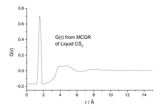
Now the fit is much better. In G(r) we have a very well defined peak from C-S pairs. This peak should have a coordination of 2 S-atoms around each C-atom. To check this use the program **coord** as shown below:
