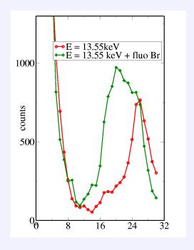
Measured counts as a function of the threshold for the diffusion in of a Br solution on both sides of Br absoption edge.
