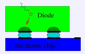
The silicium thickness  $300\mu m$  and the pixel sizes  $330 \times 330 \mu m^2$  were convenient to our beamline requirements leading to the project of buildind a new X-ray detector taking benefit of the Delphi detector peoples knowledge.
