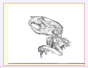
Small animal tomography: few frames (18/72) from a mouse rotated in laboratory Xray beam and the 3D reconstruction of the bones by tomography. Note that all chips have been repaired and no more defects can be evidenced.
