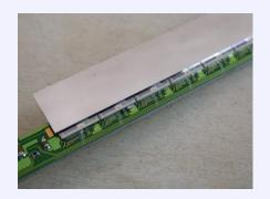
Diode  $\rightleftharpoons$  8 chips of 24  $\times$  25 pixels PCB card : drivers and regulators. Modules  $\rightleftharpoons$  acquisition card Alterra Nios kit + ethernet
