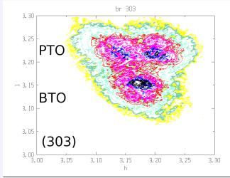
The reciprocal maps are recorded scanning the XPAD detector and rebuilt from the collected reciprocal slices. Compared to standard data collection the time can be reduced by 100. Intensity on substrate peak can reach  $10^9 \nu/s$ !
