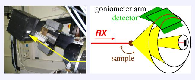
With 0-D detector pipes remove diffuse scattering, background level partly removed with conic pipes on 2d-detector.
