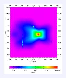
Complex shape of the diffusion around Bragg peak obtained by adding 10 (1000) frames.
