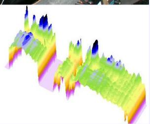
Data collection is limited by the cell apperture, which has been designed for linear detector, a few frames of 20ms around crystallisation shown at 10 frames/s during  $CaAl_4O_7$  quench.
