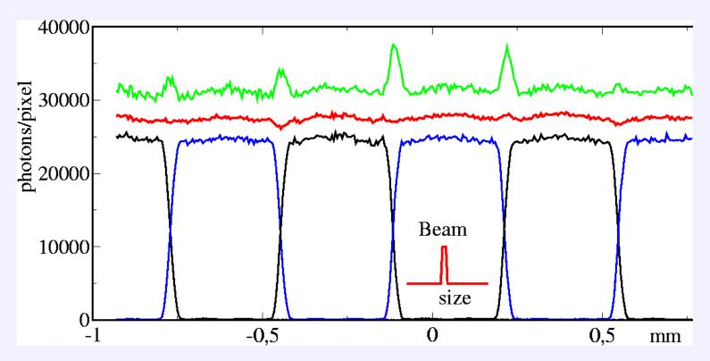
A flat field can be obtained when energies edge is perfectly adjusted in each pixel (red). In case of too low edges, this share sharing create some overcounting at pixel borders (green).
