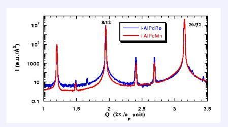
Diffuse scattering in icosaedral quasi-crystals: 7 orders of magnitude are necessary to measure this signal. Dynamic extended by **attenuators**, time consuming mapping
