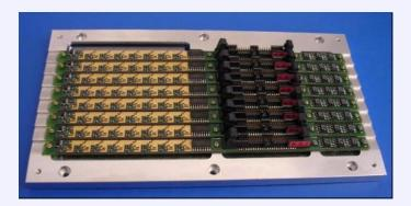
Tiled as close as possible  $\rightarrow$  reduce shading, dead zones. Metallic holder  $\rightarrow$  few  $\mu m$ . Size :  $200 \times 192$  pixels Surface  $\approx 68 \times 68 mm^2$ .
