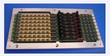
Tiled as close as possible → reduce shading, dead zones. Metallic holder  $\rightarrow$  few  $\mu m$ . Size :  $200 \times 192$  pixels Surface  $\approx 68 \times 68 mm^2$ .
