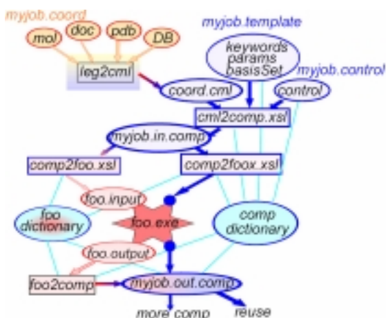
Figure 1. Computation flow for a molecule-based code, “foo”. The main XML flow is down the center, and JUMBO-based XMLization of the code is shown by blue dots. Many components are semantically enhanced by the foo-specific and the generic CMLComp dictionaries.
