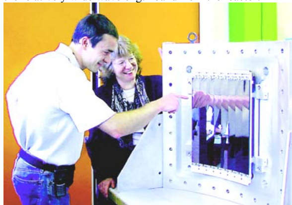
Fig. 6 A very large 2D PSD for D19, showing arrays of linear sensitive wires in front of electrodes deposited on glass (inset) 5 .
