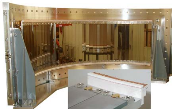
Fig. 7 The very large 2D PSD for D19, showing arrays of linear sensitive wires in front of electrodes deposited on glass (inset) 5 .
