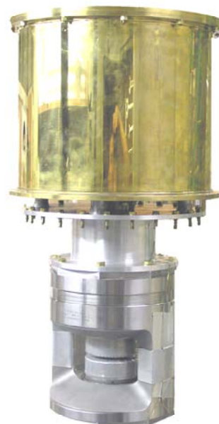
Fig. 5 The new 100 kbar pressure cell with its He cryostat 4 .
