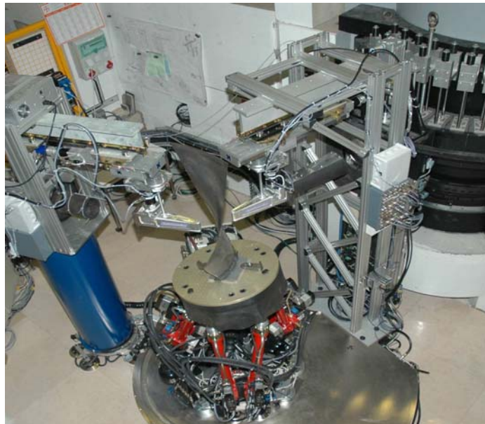
Figure 1: SALSA with an aero-engine fan-blade on the sample stage
