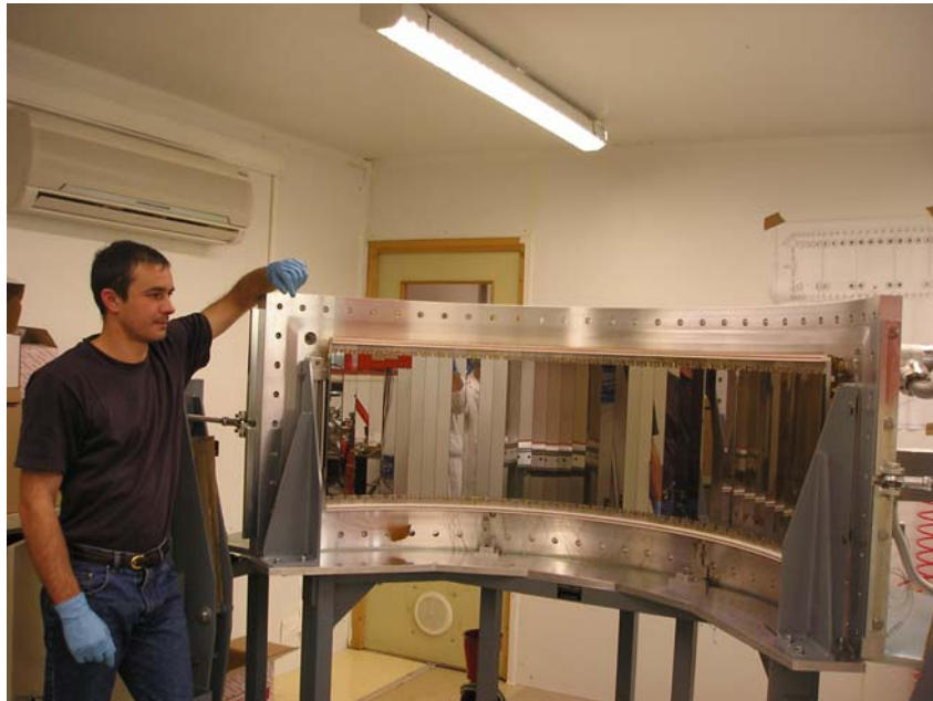
Figure 1 : the D19 banana just before closing the pressure vessel. The chrome-coated glass plates resemble mirrors from this distance. The anode and cathode wire planes are suspended a few millimeters from this surface, and seem to exert an almost irresistible attraction on the fingers of visiting dignitaries.
