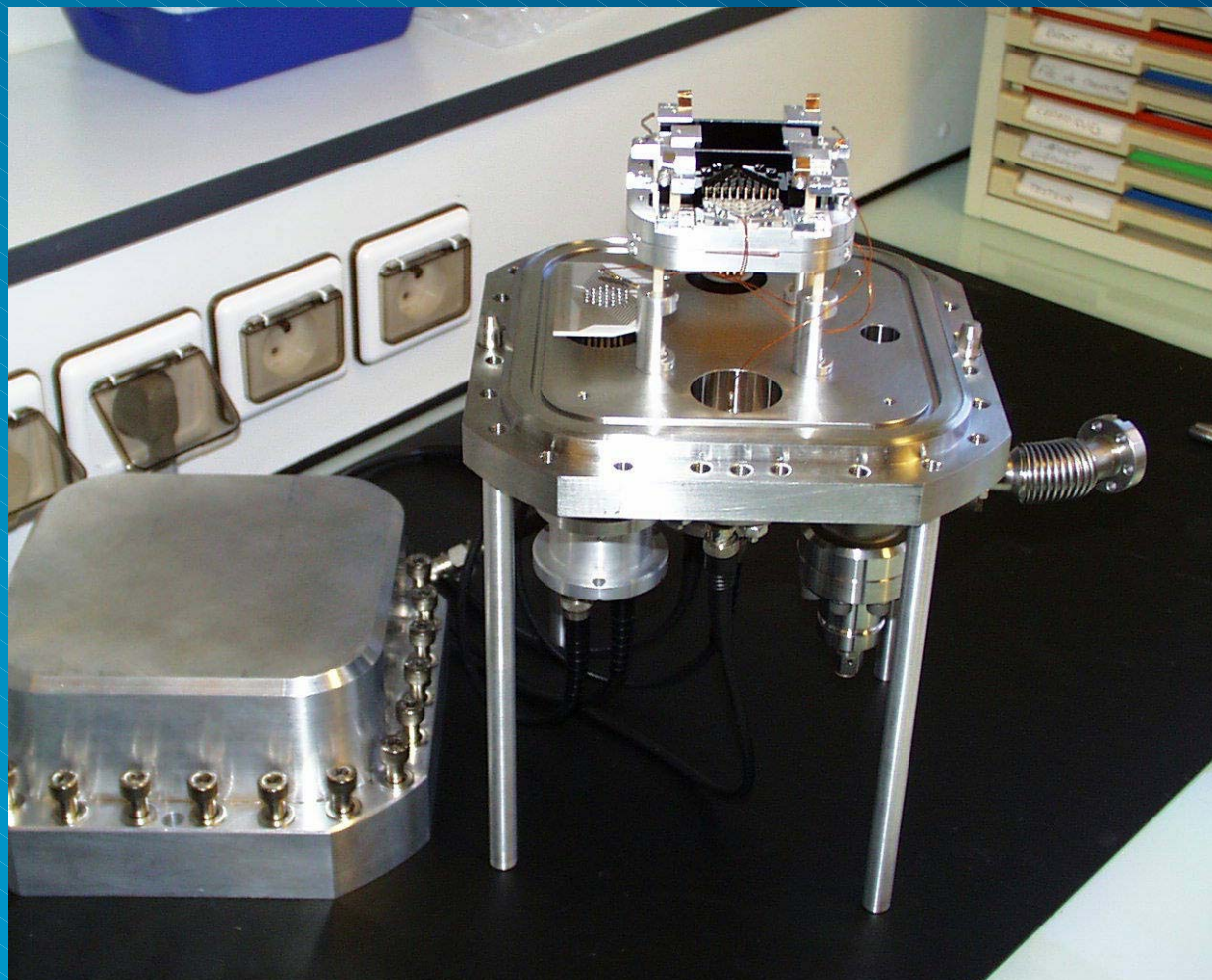
200x200 mm 2D microstrip detector for D19 fibre & protein diffractometer
